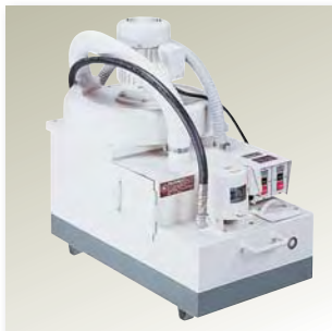
COMBINATION COOLANT & DUST EXHAUST UNIT B17-0101 Volume: 34L, Pump: 1/8HP Coolant Capacity: 20L/min Space: 15 3/4"x31 1/16" (398x798mm) Height: 26 3/4" (680mm)
